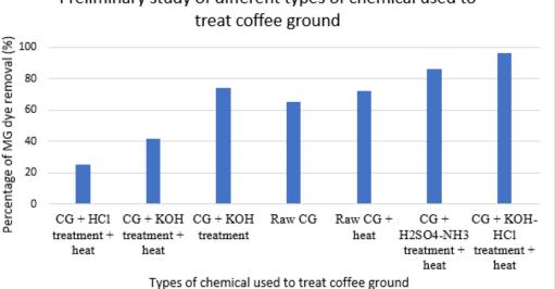
• Coffee ground treated with KOH and HCl with the heat treatment showed the highest MG dye removal percentage of 96.14 % and 23.51 mg/g of adsorption
