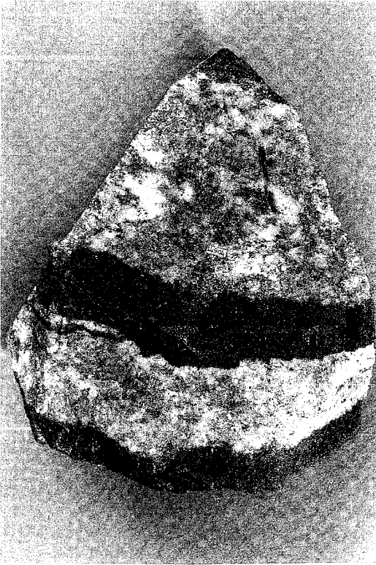
Fig. 3.2 Chromite bands in anorthosite, Dwars River Bridge, Bushveld Complex, RSA. The central band is 1.3 cm thick at the right-hand end.
